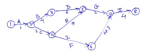
Determine the critical path and project completion time.
