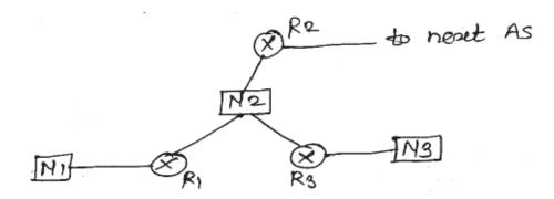
Which routers send out router link LSA and network link LSA?
