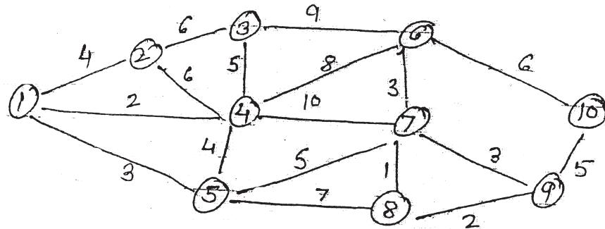
Consider the distance network. Find the minimum spanning tree of this network using the PRIM algorithm. [7]
