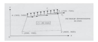
**Q5**) a) The fin shown in fig. is unsulated on the perimenter. The left end has a constant temperature of  $100^{\circ}$ C. A positive heat flux of  $q = 5000 \text{ W/m}^2$  acts on the right end. Let  $K_{xx} = 6 \text{ W/m}^{\circ}$ C and cross sectional area  $A = 0.1 \text{ m}^2$ .
