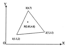
b) In a plane stress condition of a CST element shown in figure. Determine element stiffness matrix and nodal displacement. [10]
