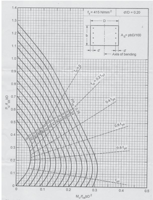
Chart No 3: Interaction chart for combined bending and compression on rectangular section with equal reinforcement on opposite
