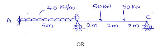
**Q4)** Analyze the frame by stiffness matrix method. Take EI as constant. Draw BMD. [16]
